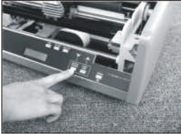
Lift the ribbon cover. Unload form.
