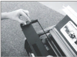
Take up slack in the ribbon by turning the blue knob counter clockwise.
