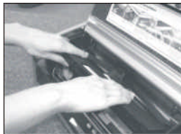
Hold the ribbon cassette with both hands with the ribbon end pointing down slightly, and insert it into the printer so the ribbon lays flat across the top portion of the noseshield.
